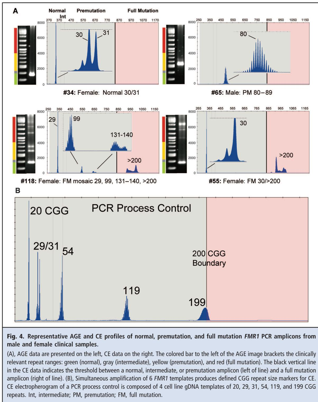
**Fig. 4.** Representative AGE and CE profiles of normal, premutation, and full mutation *FMR1* PCR amplicons from male and female clinical samples.
