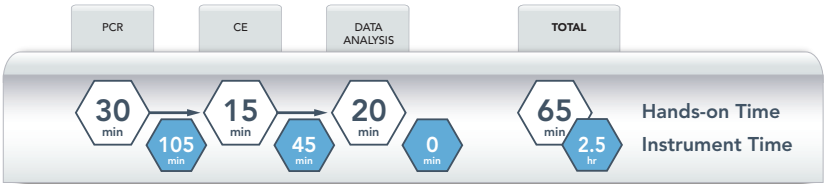
Figure 2. The DMPK PCR/CE assay workflow is streamlined from sample-to-answer. The assay can be performed with a turnaround time of ~3.5 hr for 24 samples. Total hands-on time is ~1 hr.
