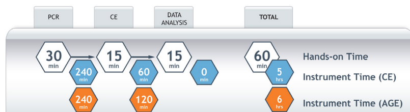
Figure 1. AmplideX PCR/CE DM1 Dx Workflow, including optional AGE workflow for larger expansions.
